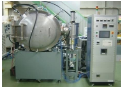
Cylindrical type large vacuum furnace
