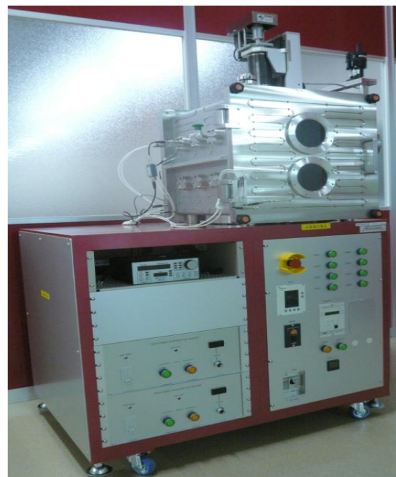
Organic 2 source Vapor Deposition System
