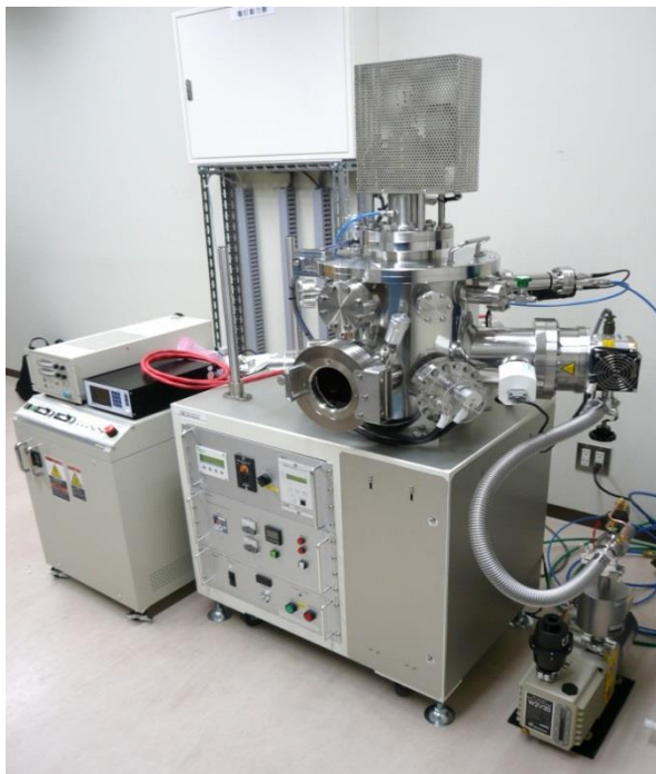
Composite Vapor Deposition Apparatus of EB heating and resistance heating
