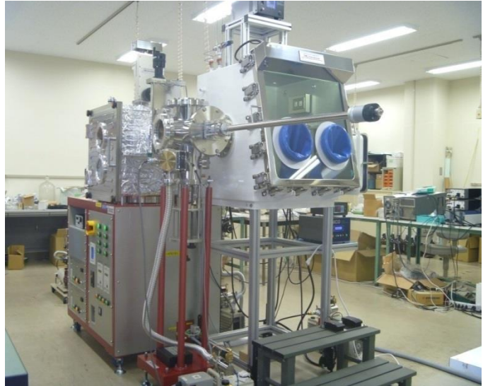
Organic Vapor Deposition System with Glove box
